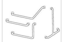
When marking out these grab rails, use centre base holes of flange protector.
