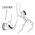
**5.** Fit grab rail into wall mount plate and tighten lock nut firmly.
