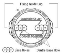
When marking out corner grab rails follow the fixing guide lug diagram shown above to suit grab rail orientation.
